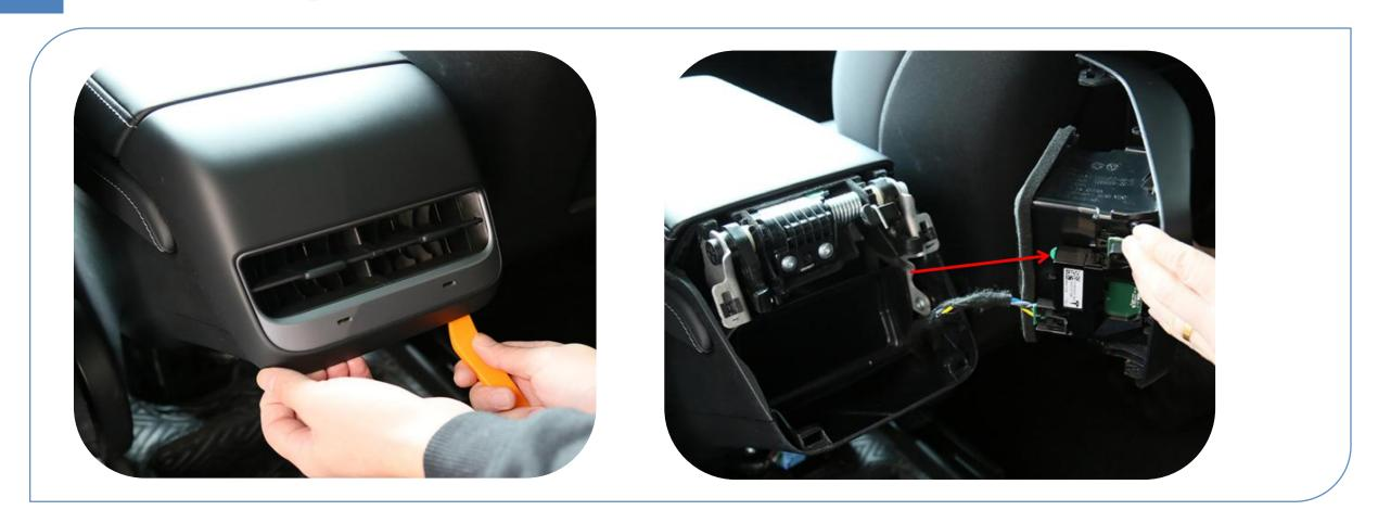
2. Use the prybar to pry open the air outlet of the original vehicle and take it off
