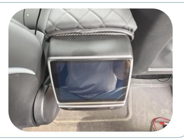
9. Place the harnesses into the area below the air outlet, and finally install the screen back to original position
