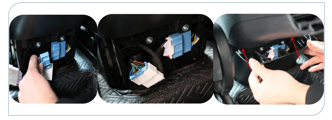
7. Turn off the power on the main screen; Unplug the blue CANbus harness of the original vehicle; Connect the white CANbus adapter plug; And then install the plastic baffle back to the original vehicle
