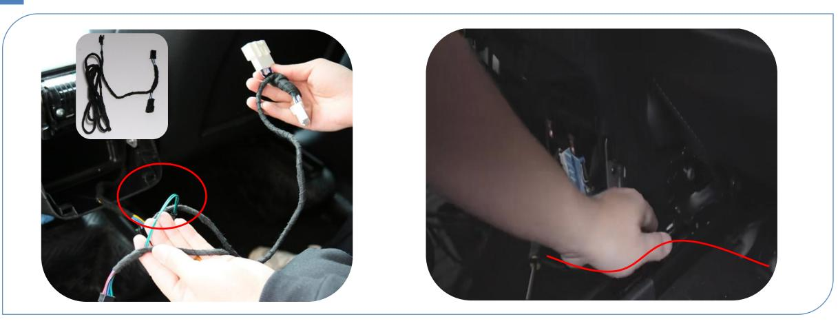
5. Connect the seat adjustment harness to the green plug, and then pull the harness to the passenger seat
