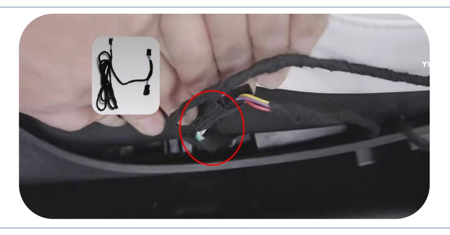
6. At the side of the rear co-driver, pry off the seat adjustment baffle with a pry plate and pull off the plug, then connect with the adapter plug.
