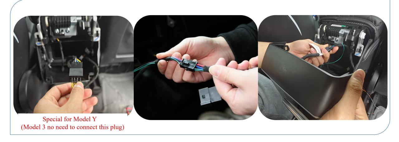
8. Take out the 7.2" screen in the packaging box and plug in the power cable and USB charging control cable of the screen respectively. Remove the built-in clips and first attach the screen frame from the top, then attach it from the bottom
