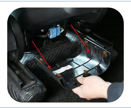
1. At the bottom of the rear vent outlet, pry open and remove the plastic baffle
