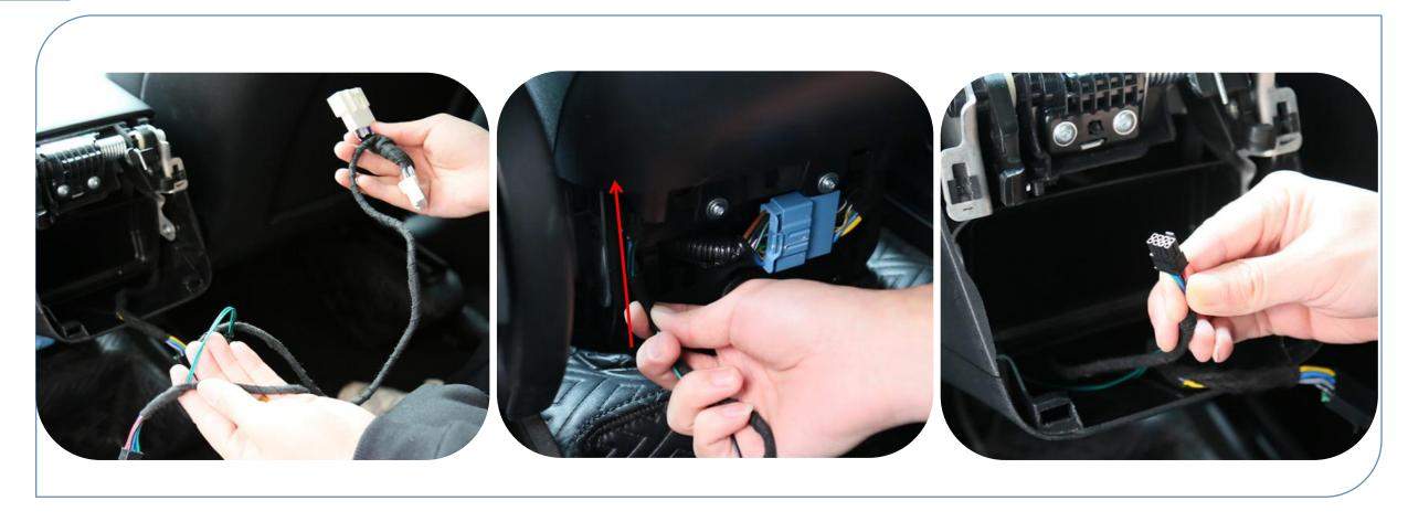
4. Take out the harness in the packaging box, put the black interface through the gap at the bottom left of the airoutlet, and pull it out from above
