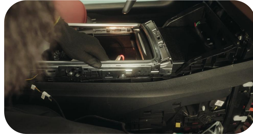
33. Install the chrome plated strip and tighten the fixing screws.
