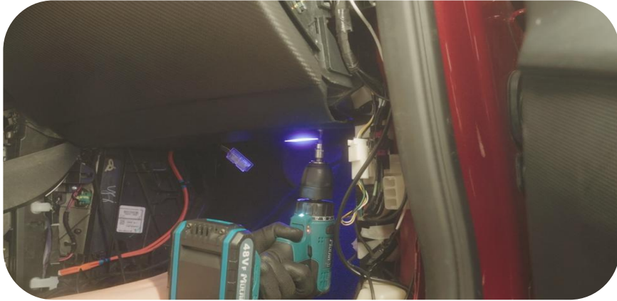
17. Remove the instrument lower guard plate
