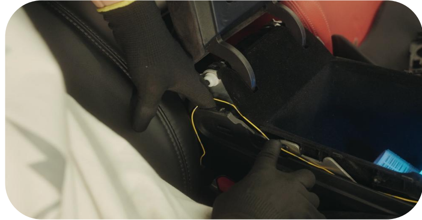
29. Run Line 2 along the edge of the saddle to the rear air outlet.
