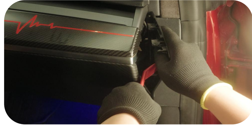
14. Remove the triangle plate
