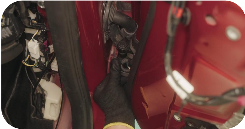
56. Both ends must be opened (Be sure to press back after finishing the line, otherwise water will enter)
