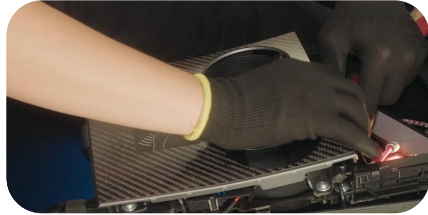
6. Remove the identification card door panel (note that there is a plug inside)
