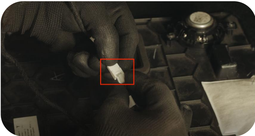
50. 36 to 36 , right front footwell light plug docking
