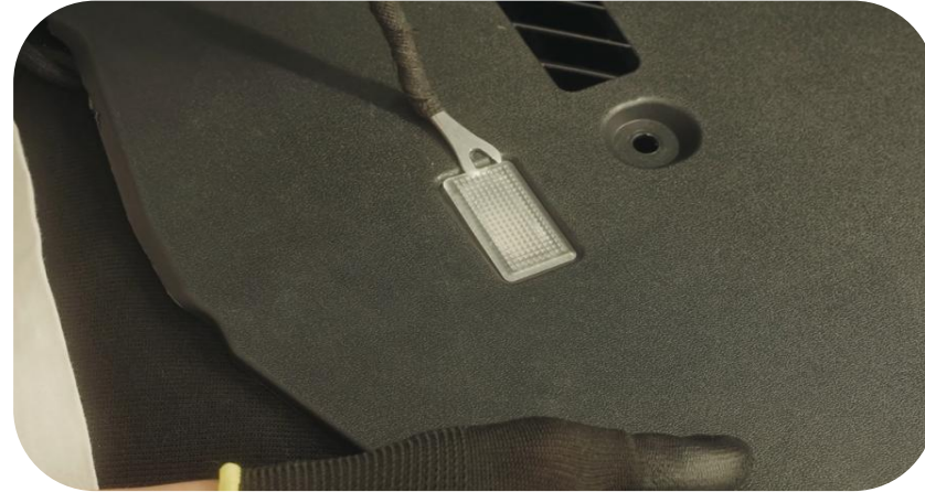
49. Pry open the footwell lamp on the lower trim panel of the glove box and replace it with the footwell lamp that comes with the product.
