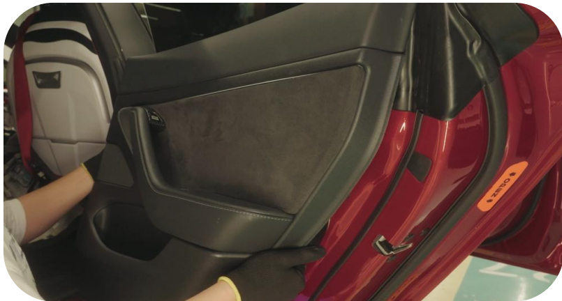
78. Remove the rear door panel
