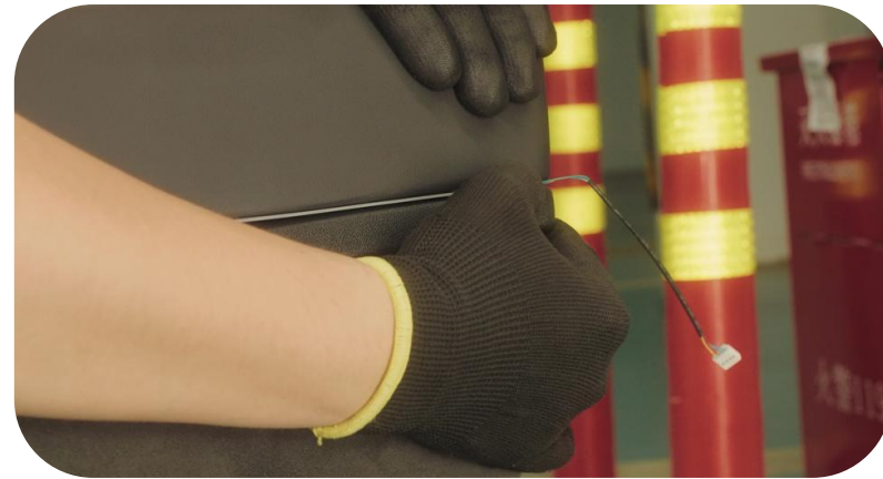
87. Press the ambient light strip into the gap in the rear door panel.
