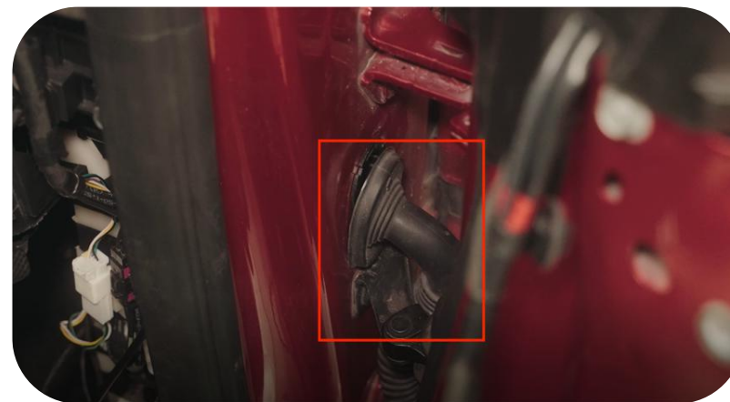
55. Open the door and the wiring harness drain pipe of the body
