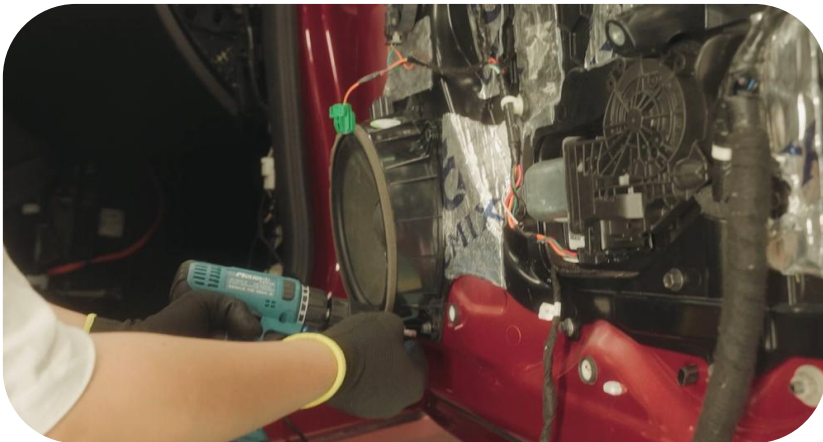
54. Remove the speaker fixing screws and remove them
