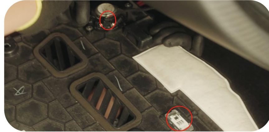
18. Unplug the footrest lamp plug and speaker plug in the guard plate
