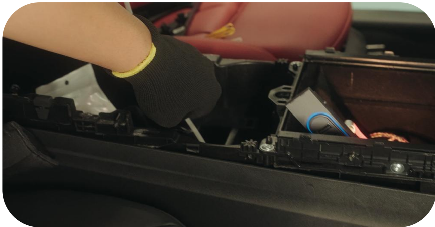
19. Thread the threading strap from the cup holder to the saddle side plate.
