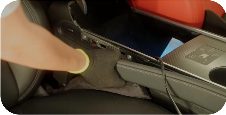
1. Remove the saddle trim panel
