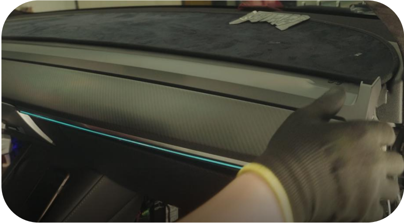
48. Install the instrument trim panel
