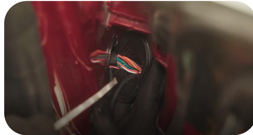
57. Use a threading tape to thread it from the top
