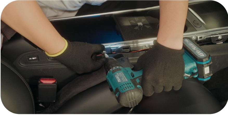
5. Unscrew the fixing screws on the left and right sides of the saddle chrome strip
