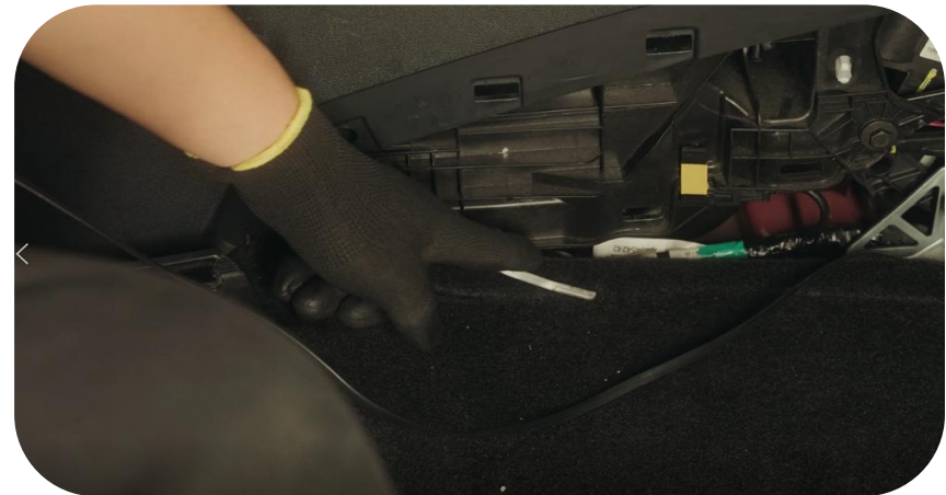
19. Thread the threading strap from the cup holder to the saddle side plate.
