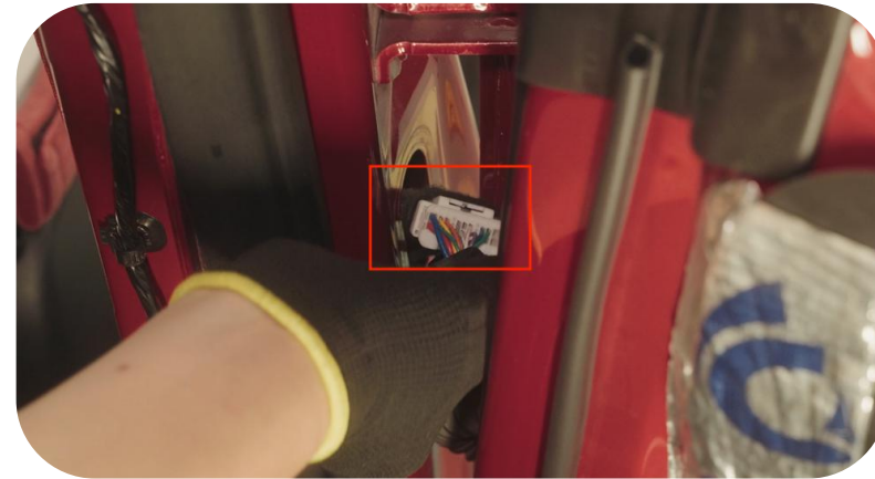
79. Unplug the main plug of the door harness inside
