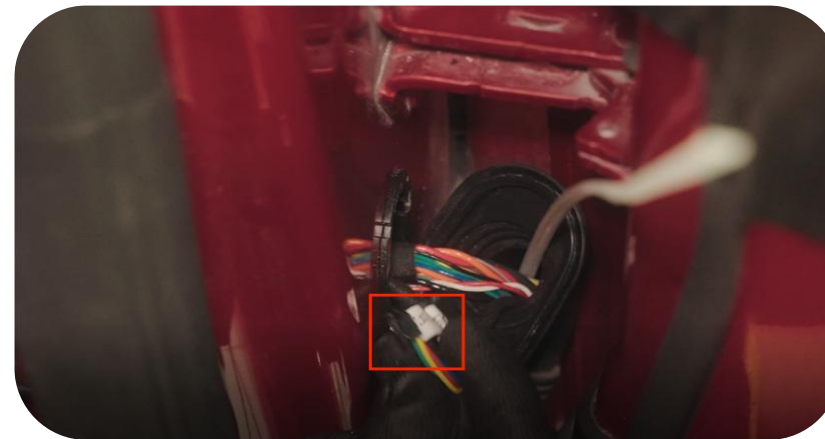
59. Move the 22 label plug from the car body to the top of the waterproof pipe in the picture
