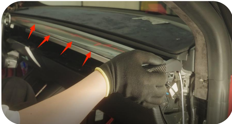
38. Run the wiring harness along the edge to the lower side panel.
