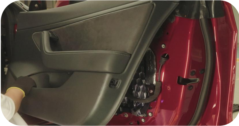
52. Pull open the door panel
