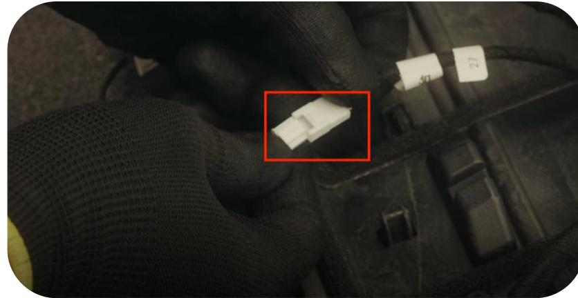
43. 29 to 29 , dashboard ambient light docking
