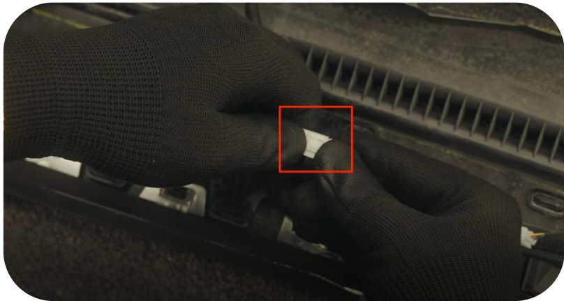
42. No28 to 28 , dashboard ambient light docking
