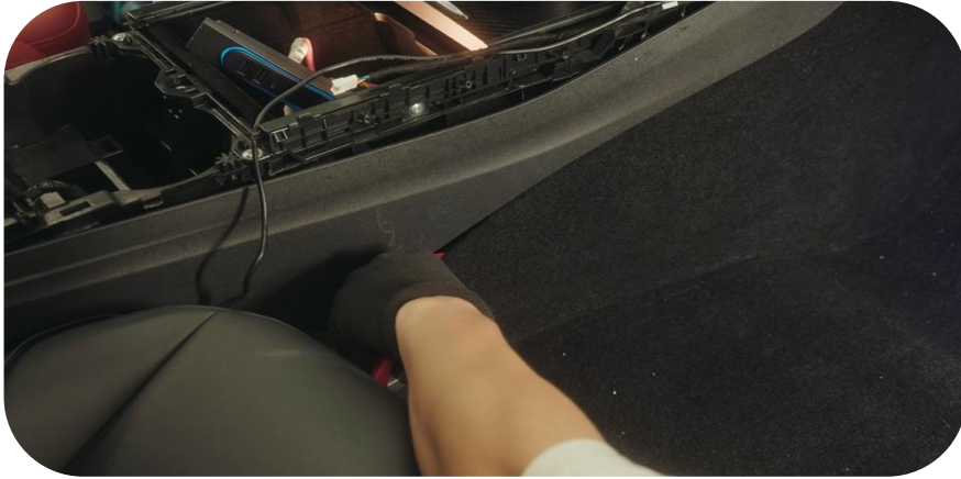
13. Remove the saddle side guards
