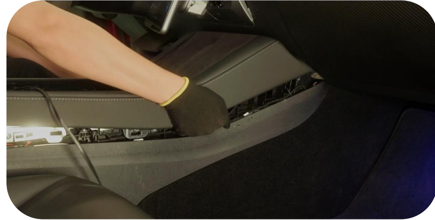
2. Lift up the wireless charging panel (Note that there is a wireless charging plug inside)
