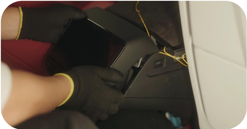
30. Unplug the rear saddle air outlet
