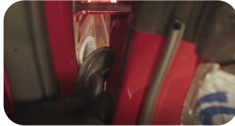
77. Remove the water pipe between the rear door and the body
