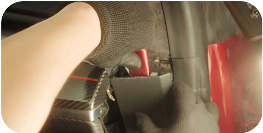
15. Remove the rectangular trim panel
