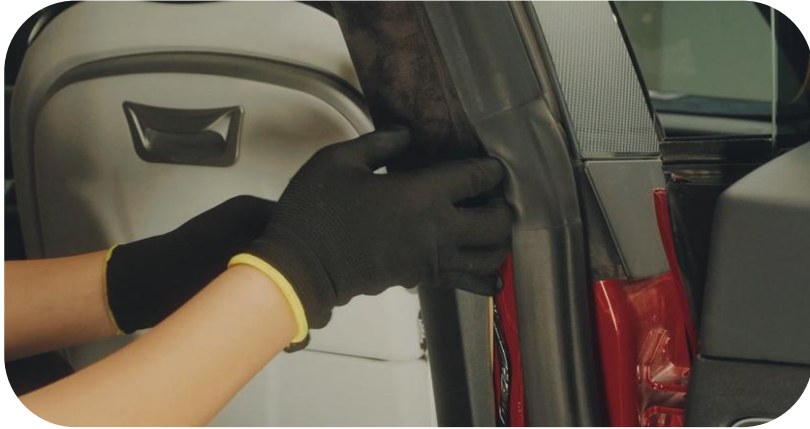
76. Remove the upper and lower trim panels of the B-pillar
