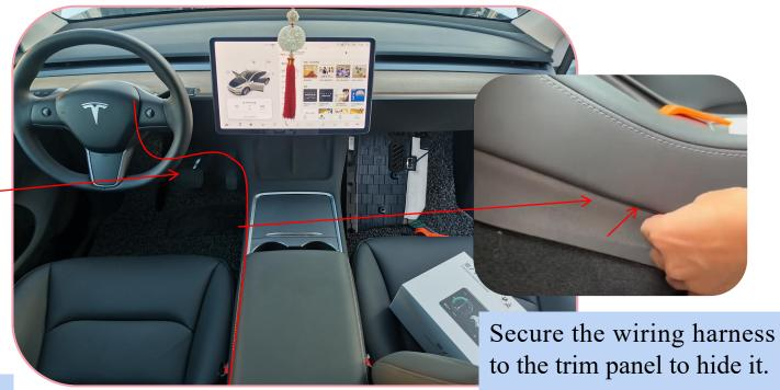
Wiring harness routing diagram
