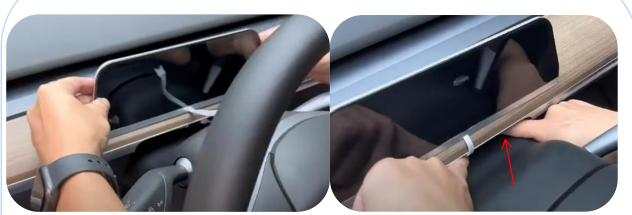
6. Tear off the 3M adhesive, position it in the center, connect the plug, and then conceal the plug.
