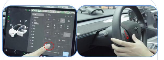
5. Adjust the control settings by lowering the steering wheel to its lowest position and turning it all the way to the left
