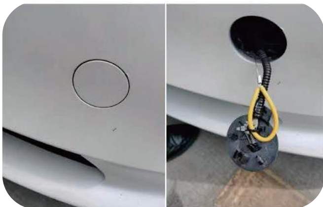
16. Fixing position of emergency cable After prying off the trailer cover of the front bumper, tie the emergency cable to the trailer cover with a tie (see the position in the picture)
