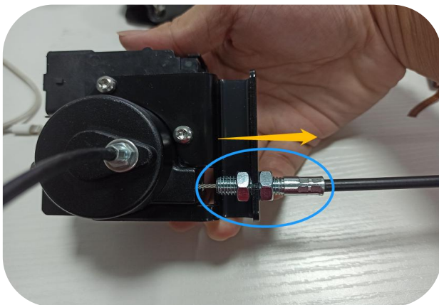
9-2. Install the electric suction lock If step 9.1 cannot be adjusted, adjust the screw at the lock motor and turn it to the right to loosen it
